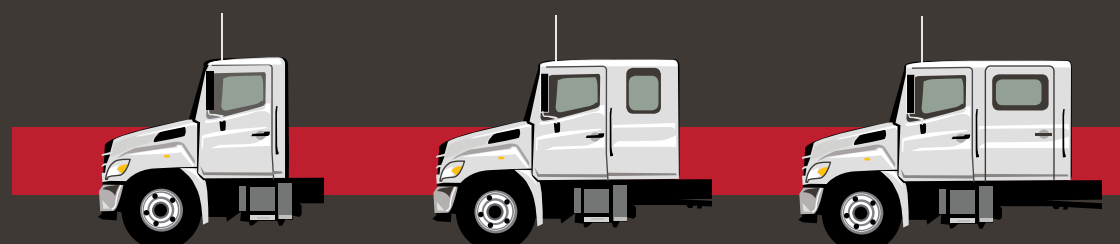
DAY CAB (Seats 3) BBC: 108" EXTENDED CAB (Seats 5) BBC: 138" CREW CAB (Seats 6) BBC: 152.8"
